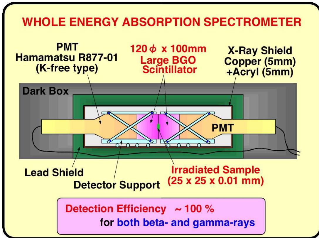
Figure 1: Whole Energy Absorption Spectrometer WEAS set-up
