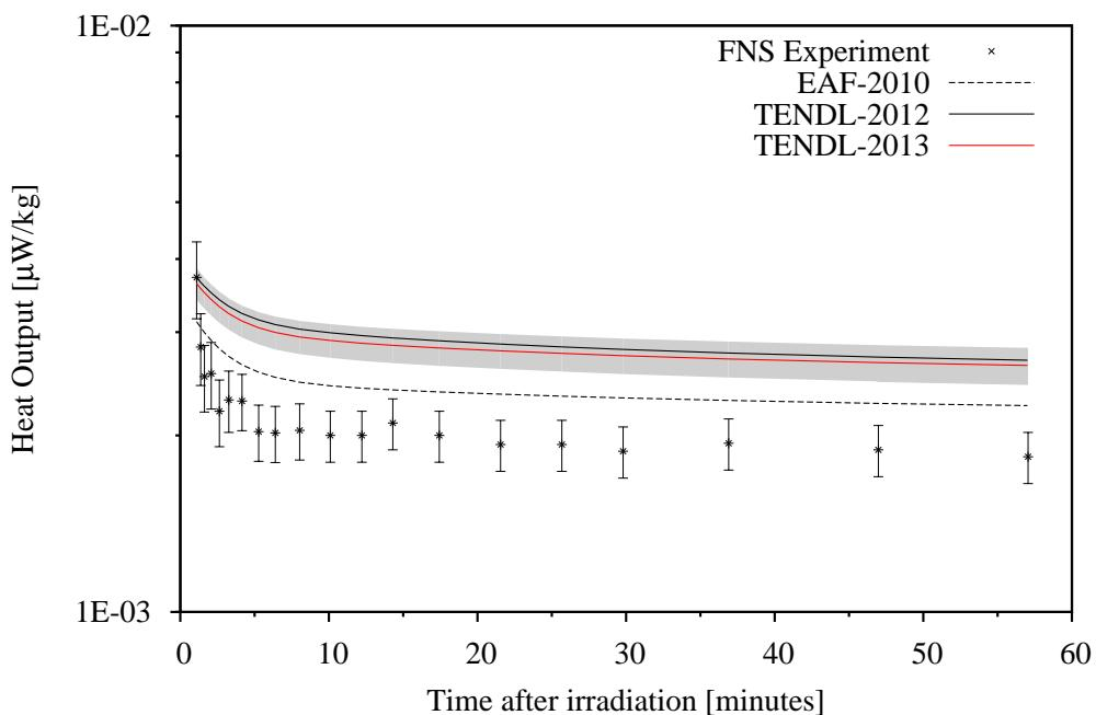
Rhenium: there is quite good agreement to the newer experimental results for this element with EAF-2010, nearly within the experimental uncertainties. However, the experimental result from the 1996 batch is significantly different. This could be due to the rarely observed shadow or iceberg effect. Furthermore, Re188 response is over-predicted by TENDL's libraries, shadowing the Re186 one. Effect seen in the next page Log-Log graph.
