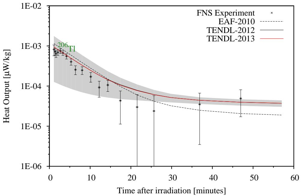
For Bismuth, some large differences and uncertainties can be seen between the two experimental data-sets. This is also the case in the predictions derived from the different databases.
