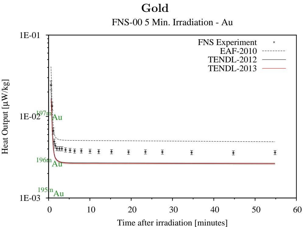
Gold: from such a picture above one may deduce that there could be an over-prediction with EAF-2010 of the heat generated by the Au196n isomer at a level of about 30%. However, Au196n production paths are lacking in the TENDL libraries.
