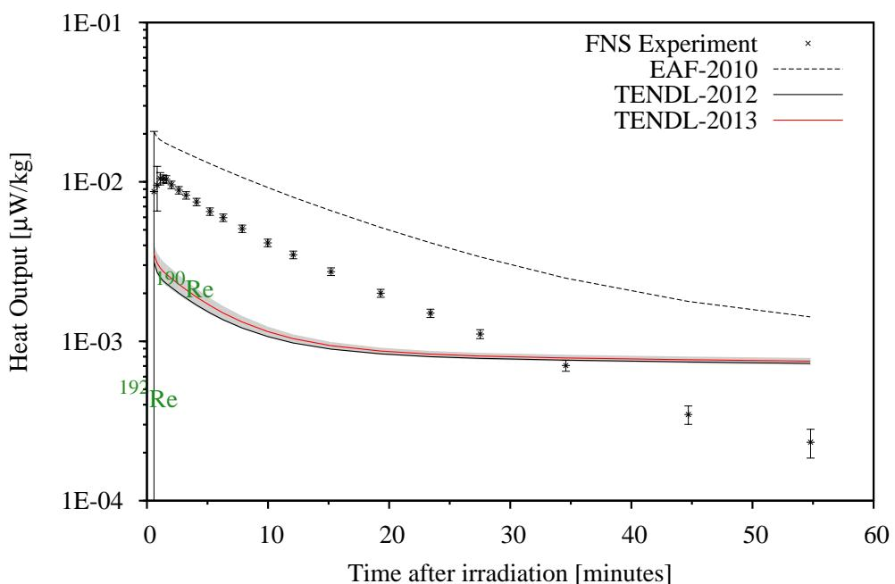
For Osmium, here again the correction made on a grossly overestimated ( $n,n'$ ) channel provide a better estimate of the heat output levels (compared with EAF-2010), although major disagreement still exists between databases for both the isotopic contributions and their heat-output levels. TENDL's libraries are lacking production pathways for Os190m.
