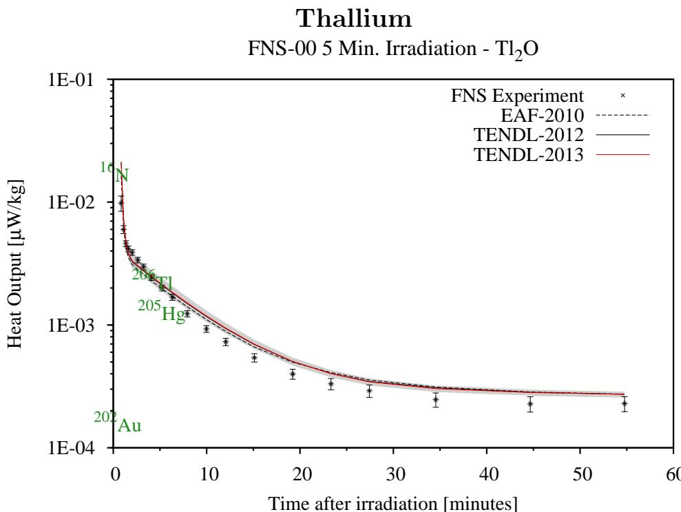
For Thallium, an excellent agreement can be seen when the TENDL-2013,-2012 or EAF-2010 databases are used. TENDL-2011 [12] performed poorly.
