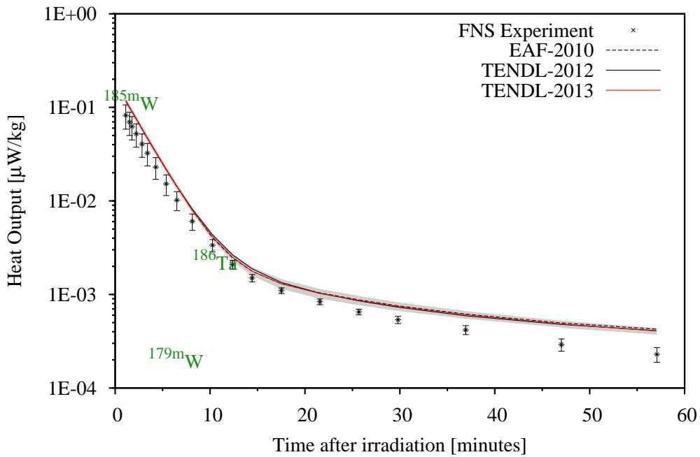
For Tungsten, a better than expected level of agreement is observed for this particularly troublesome, in nuclear data terms, element. The systematic code over-prediction on both batches (although by more in the 2000 case) may need to be addressed via an in-depth analysis of the two production routes involved.
