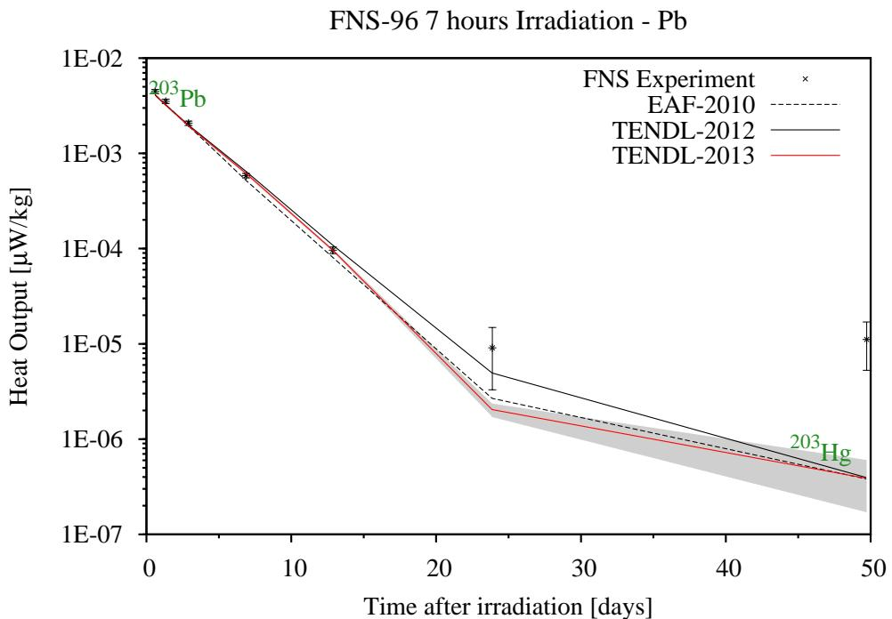
A good agreement is seen in the above graph, although large discrepancies and uncertainties occur in both the measurements and TENDL's results beyond 20 days of cooling.
