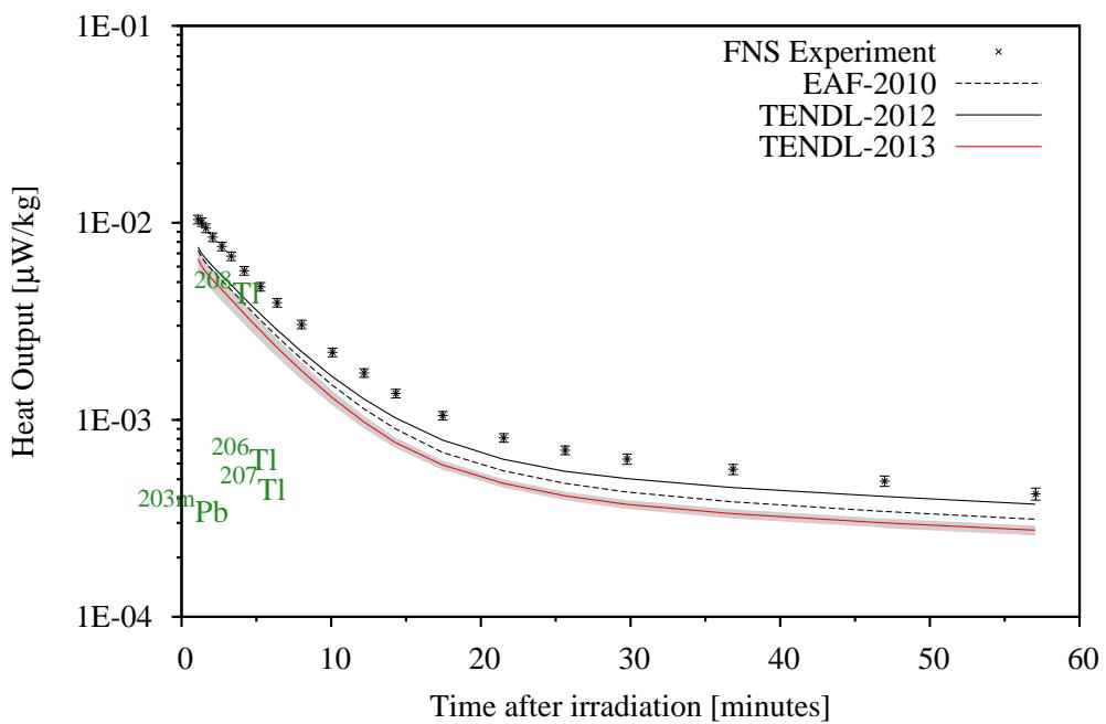
For lead, the experimental data sets are somewhat different, although the more recent one seems better predicted by the calculations, particularly at longer cooling times. However, in both batches the short term heat predictions seem to be low compared with the measured ones.
