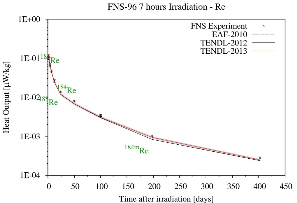
A much better agreement, compared to the 5-minutes analysis, is seen from half a day up to more than a year of cooling. Note in this case the unusual case of metastable isomer having a half-life greater than the ground (Re184m vs. Re184).
