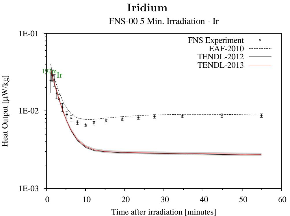
For Iridium, a most interesting experimental decay heat shape can be seen, underpinning an increase in heat due to the presence of an isomeric daughter with a half-life shorter than the parent, coupled with a potent decay heat. TENDL's libraries are lacking the Os190m and Ir192n production pathways that are present in EAF-2010. Note that along the direct ( $n,d$ ) production route for Os190m there is also a decay path from the long-lived Ir192n.
