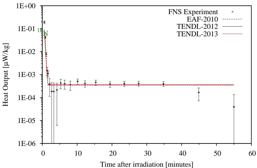
For the lanthanide Thulium, the representation of the experimental data is not too bad, allowing for the large experimental uncertainties at short and long cooling times, and the possibility of some missing isomers in the calculational paths.
