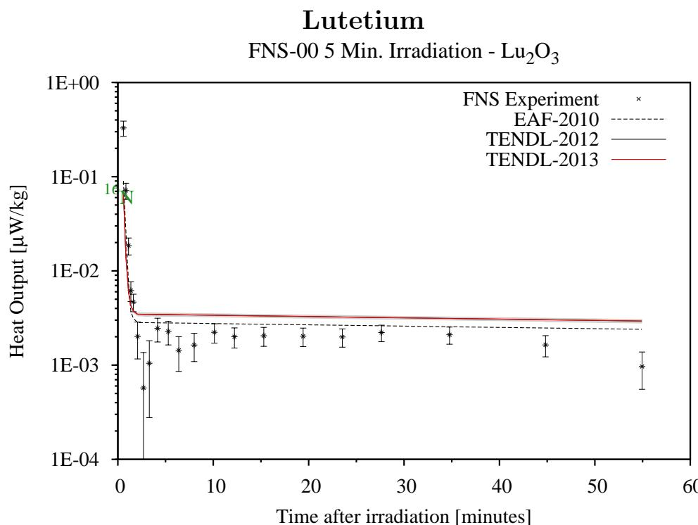
For Lutetium, once again the experimental results in the minute ranges show some structures, possibly underlying a lack of isomeric state and associated decay data, or an incorrect level of the subtracted tape contribution.
