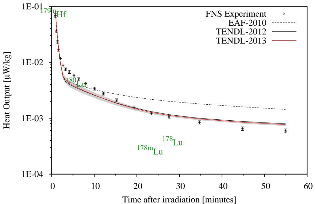
For Hafnium, the analysis of this element with anterior databases was extremely poorly interpreted because of a gross overestimation of the  $\text{Hf}^{177}(\text{n},\text{n}')$  channel. With this overshadowing effect now taken out one can still observe half life and/or branching ratio inconsistencies, but TENDL's libraries shows a significant improvement over the earlier databases.
